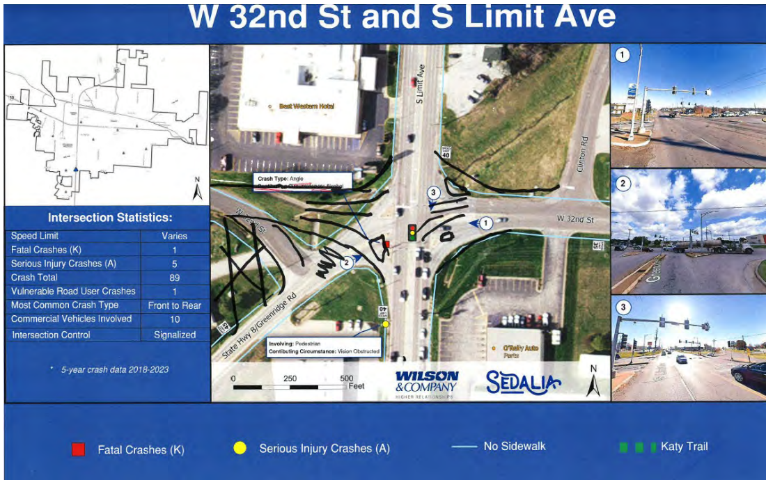
Figure 3 - Figure 6 - Intersection (32 St and Limit Ave)
